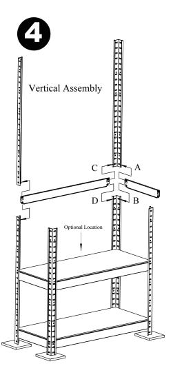
This unit can be assembled upright (vertically) or side-by-side (horizontally).
